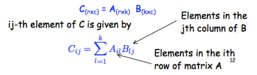
Outer indices given dimensions of resulting matrix, with r rows (A) and c columns (B)  $C_{(rxc)} = A_{(rxk)}^{\prime} B_{(kxc)}^{\prime}$
