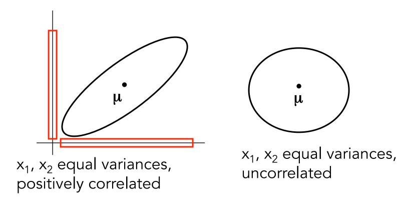
**Eigenstructure** (the eigenvectors and their corresponding eigenvalues) determines the geometry of **V**.
